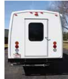
Rear Wall (shown with optional rear door & center brake light)
